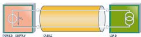
Fig. 3: DART Power Circuit: Intentional simplicity – comprising a power supply, cable, and consumer load. Can be easily adapted to a wide range of requirements.
