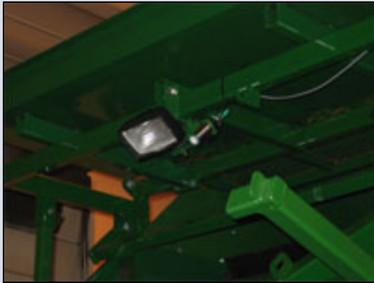
Fig. 2: Level measurement using the ultrasonic sensor UB2000-30GM-E5-V15
