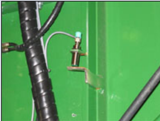
Fig. 3: Determining the position of the casing using the NBB8-18GM50-E2-V1 inductive sensor
