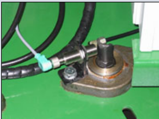
Fig. 4: Counting the revolutions of the axle with the NBB8-18GM50-E2-V1 inductive sensor
